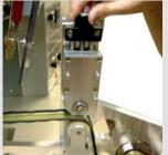
KIT Longitudinal zipper cutter - continuous cut for taped zipper
