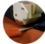
Machine for joining two fabrics. An adhesive tape has to be applied to the edge previously. The machine is fitted with an additional heater and a blade nozzle to heat the area inside the joint effectively. The purpose of this machine is to eliminate the long fusion press step.
